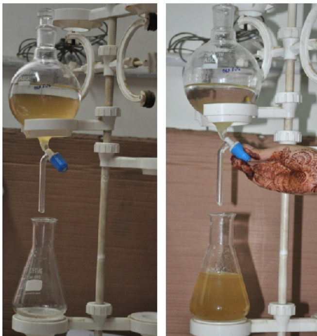
Fig.4. Solvent Extraction set up for microbial cell free culture extraction.
